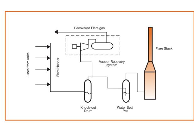
Figure 4: Simplified flow diagram for a flare system
